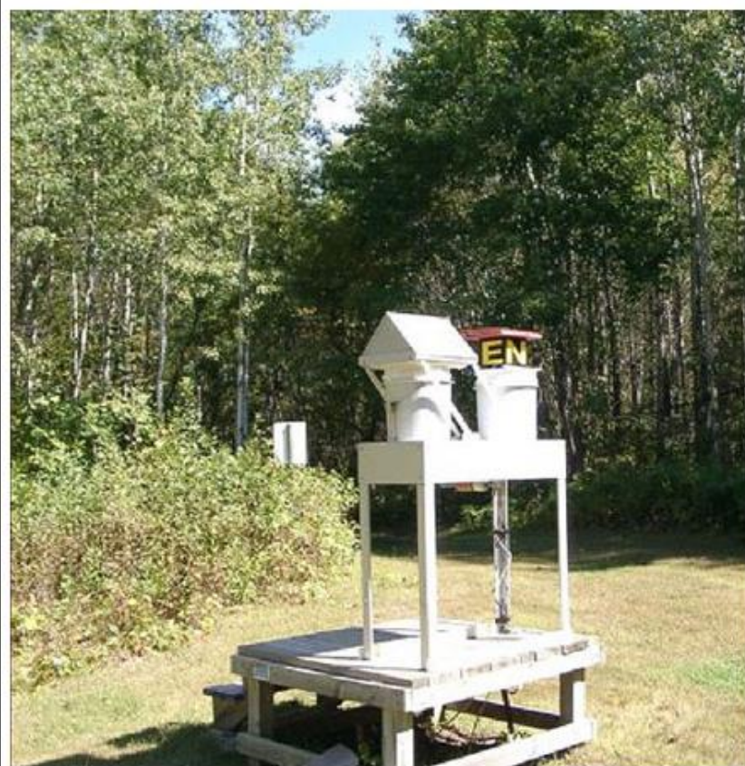
Figure 20. Collector used for trapping Phakopsora pachyrhizi spores in rainwater. (Image from National Atmospheric Deposition Program, http://nadp.sws.uiuc.edu/ , copyright-free)
