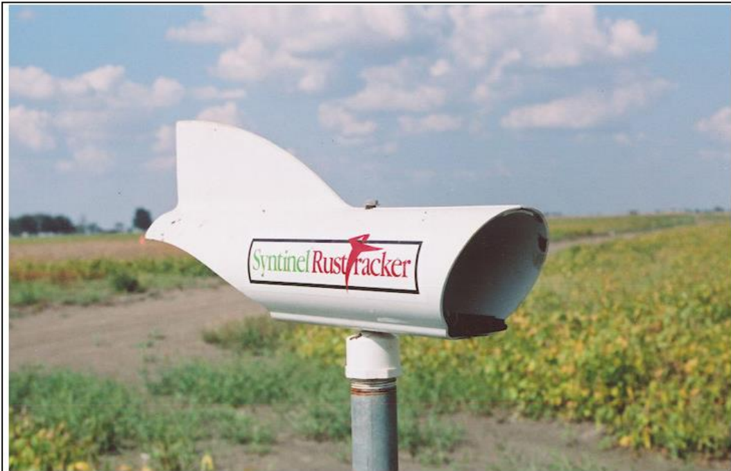
Figure 19. Spore trap used for the detection of rust-like spores. (Photo by J. Rupe)
